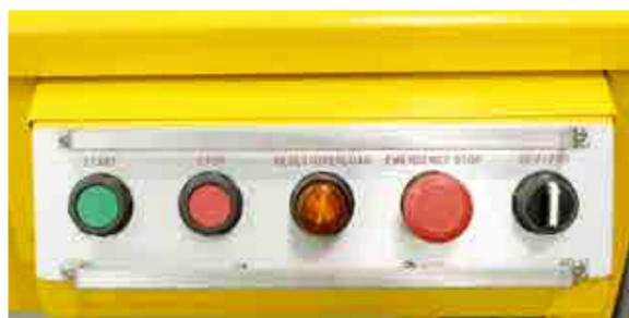
The control panel is conveniently located at the front of the machine therefore alleviating any risk that can be caused by having to lean over to control the machine which can lead to articles of clothing being caught by moving parts leading to possible injury.
